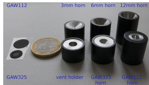
Figure 2. The different acoustic vents and horns tested, as well as the vent holder. 1 EUR coin for scale.
