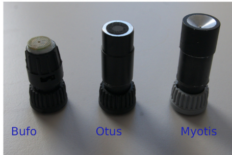
Figure 6. Recommended microphone designs: the minimalist Bufo, the silent Otus, and the allrounder Myotis.
